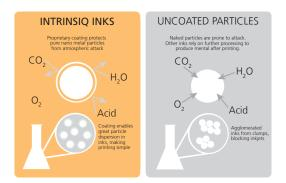
Production of these conductive structures using low cost, high throughput printing technologies enables rapid production of electronic components, on a wide variety of substrates. Copper nanoparticle production is achieved using plasma technology and supplied as pastes or inks for use in screen and inkjet printing. Curing of the copper yields in 5 to 10 times bulk resistivity and can be either performed by laser processing or using reducing atmosphere at elevated temperatures.
