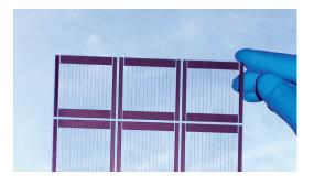
Processing of the inks is performed by inkjet and screen printing. Line widths down to 30  $\mu$ m at heights between 200 nm and 1  $\mu$ m have been achieved by inkjet printing and processed as grid structures to replace ITO as transparent electrode. Processing of OLEDs and OPVs on such grid structures could be performed by overcoating the grid or after embedding it in an inert resin.
