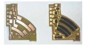
For PCB and RFID applications the cost factor is very crucial for the commercialization of any product. Therefore material and processing costs need to be competitive with alternate processing techniques. Inkjet printing and laser curing on R2R facilities offer a competitive technology for the processing of RFID labels on various substrates such as PET or paper.
