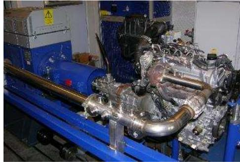
3 fully equipped engine benches for emissions testing
