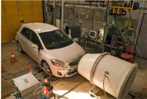
Chassis dyno for vehicle emissions testing
