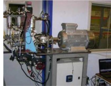
Fuel injector test rig
