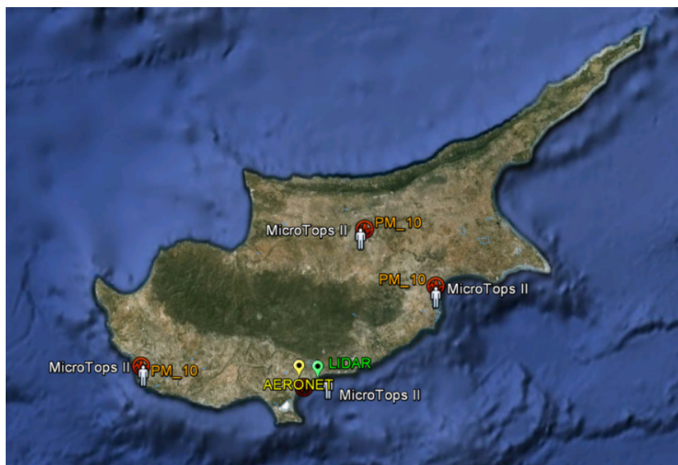
Figure 8. Overview of the available instrumentations at the selected sites within AIRSPACE project. Limassol was the main site (LIDAR, AERONET, PM), Nicosia validation site (MicrotopsII, PM); 15-day campaigns were conducted at Larnaca and Paphos.
