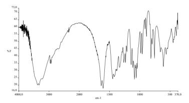
Fig. 1. FT-IR spectra of 1 in KBr
