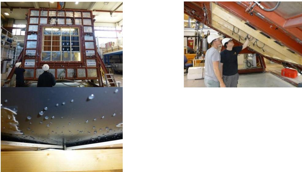
Fig.1. Large-scale laboratory wind-driven rain tightness testing of BIPV applying a rain and wind box. Comparing BIPV tiles with normal tiles (left), inspecting for any water leakages
