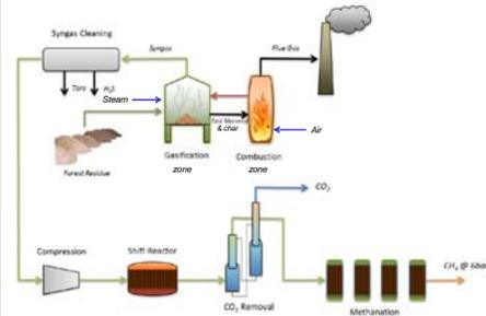
Fig. 2 Simplified schematic of GoBiGas 20 MW<sub>SNG</sub> demo plant Gothenburg Sweden [1]
