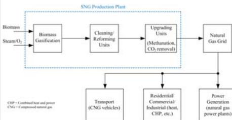
Fig. 1 BG-SNG plant and applications block diagram
