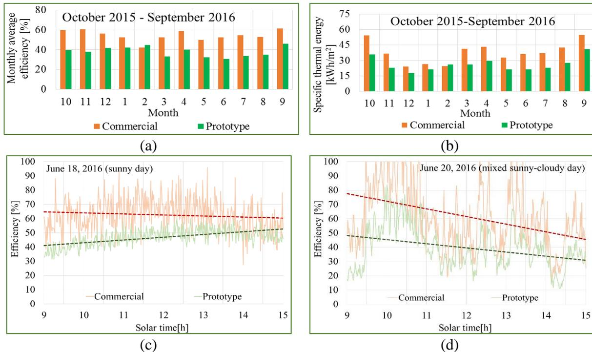
Fig. 1. (a) Average monthly solar to thermal conversion efficiency and b) monthly solar output over one year; (c) typical conversion efficiency during a sunny and (d) a mixed day for the commercial collector and prototype, vertically installed in outdoor conditions
