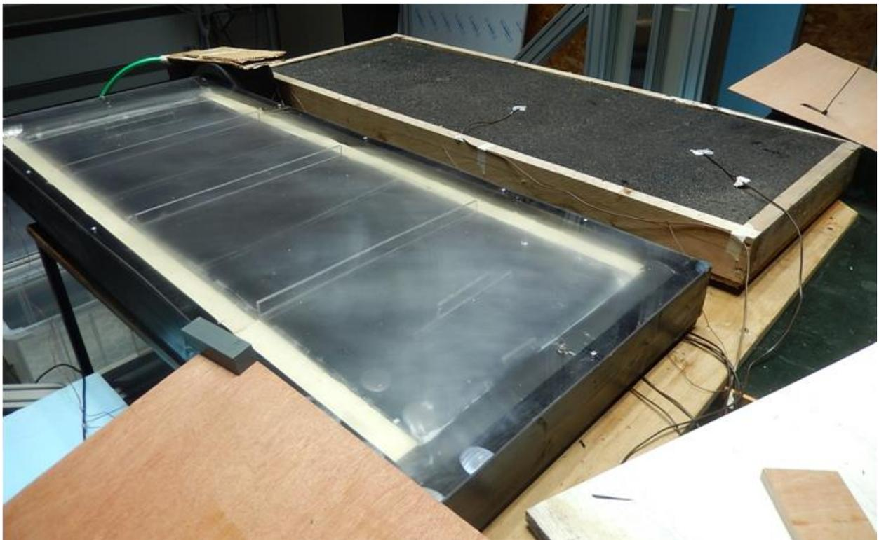
Figure 1: Senergy PCNT (left) and ACNT (right) solar water heating collectors
