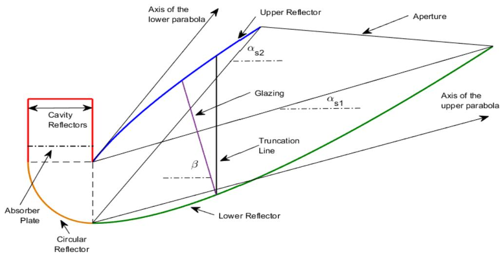
Fig. 2. Solar collector cross section
