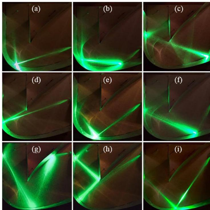
Fig. 10. Ray tracing using a laser for three solar altitude angles:  $17^\circ$  in (a), (d) and (g);  $39^\circ$  in (b), (e) and (h);  $60^\circ$  in (c), (f) and (i)
