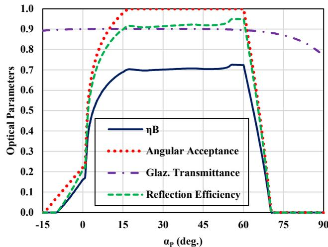
Fig. 8. Optical parameters versus solar altitude angle
