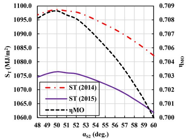
Fig. 5.  $S_T$  and  $\eta_{MO}$  versus angle of the lower parabola axis. Glazing inclination of  $66^\circ$
