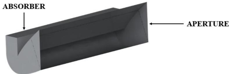
Fig. 1. Isometric view of the IACPC collector to be designed
