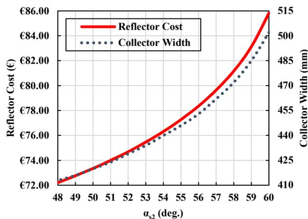
Fig. 6. Reflector cost and collector width *versus* angle of the lower parabola axis.
