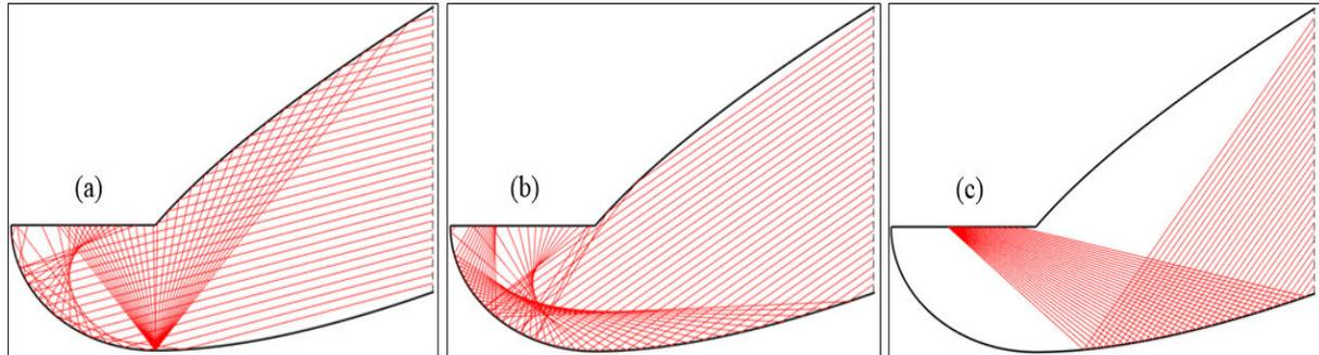
Fig. 9. Graphic results of ray tracing for solar altitude angle of (a)  $17^\circ$ , (b)  $39^\circ$  and (c)  $60^\circ$
