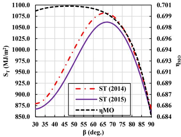
Fig. 4. Total absorbed energy and mean optical efficiency versus glazing inclination
