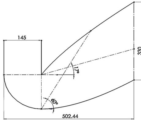
Fig. 3. Collector's initial design (mm)
