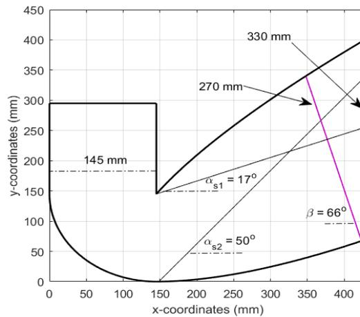
Fig. 7. Cross section with dimensions of the solar collector to be fabricated
