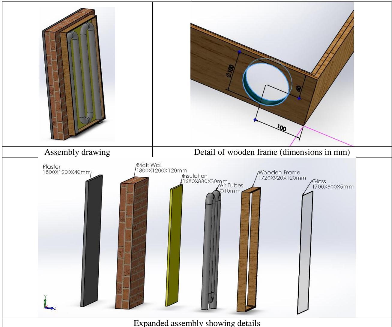
Figure 1. Integrated hot air collector utilising an aluminium foil duct
