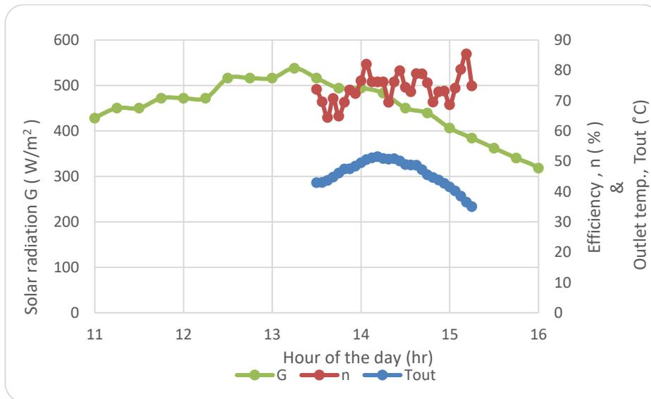
Figure 8. Efficiency of the integrated hot air collector with internal metal separators, varying during the testing period, from a minimum of 63 to a maximum of 82%.
