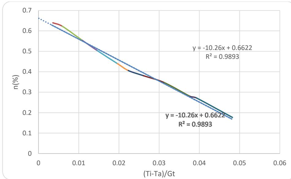
Figure 7. Efficiency of the integrated hot air collector utilising an aluminium foil duct, with a fun speed of 1.9 m/s and an incident radiation of 560 W/m<sup>2</sup>. Abbreviations: n= efficiency, Ti= initial air temperature (°C), Ta= air temperature of environment (°C), G<sub>t</sub>= solar radiation (W/m<sup>2</sup>)
