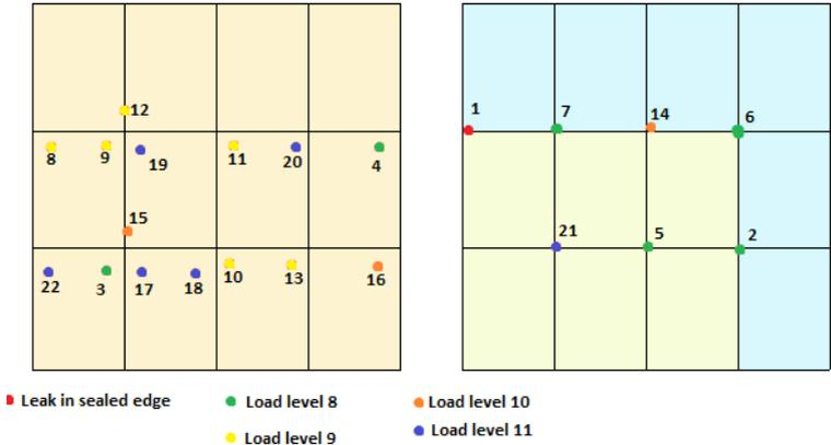
Fig. 13. Leakage points observed during rain tightness test of BIPV roof tile at 15 degree inclination (Andenæs, 2016).
