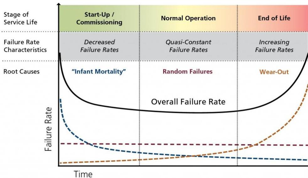
Fig. 7. The “Bathtub curve” of failures occurring in solar PV modules (Sirkin, n.d.).
