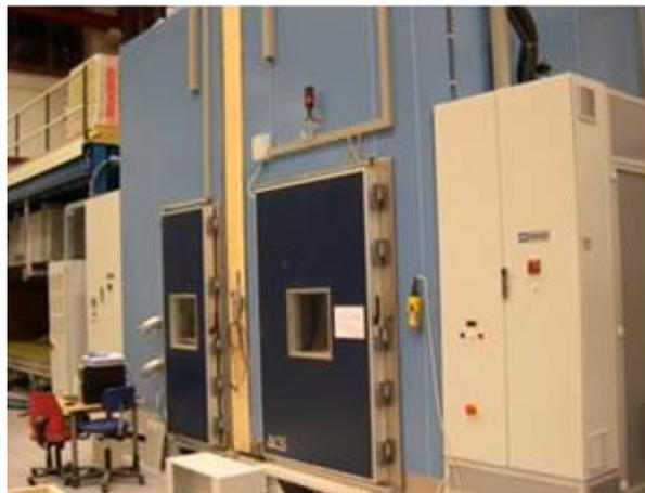
Fig. 3. Specially customized large-scale vertical building envelope climate simulator consisting of a sample field installed between the exterior and interior climate chambers (Jelle, 2013).
