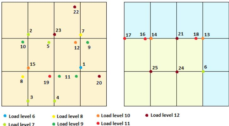
Fig. 12. Leakage points observed during the rain tightness test of the BIPV roof tile at a 30 degree inclination (Andenæs, 2016).
