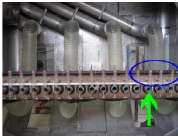
Fig. 5. The boom inside the RAWI box which delivers wind-driven rain across the sample area. The blue tubes on top (blue ellipse) supply water down to the transparent vertical cylinders (blue ellipse) where it hits the air stream that blows out of the air tubes (green arrow) and is blown onto the sample area (Breivik et al., 2013).
