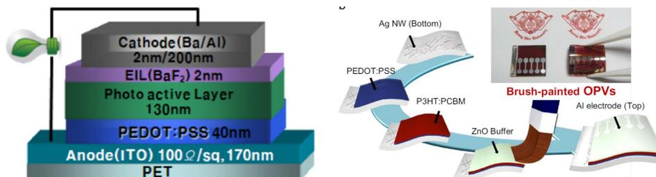
Fig. 6. (Left) Device structure of a flexible polymer solar cell (Heo et al. 2011). (Right) Schematics depicting a brush painting process of preparing brush-painted flexible organic solar cells. The inset photo shows the flexibility of the brush-painted flexible organic solar cells (Kang et al. 2014).
