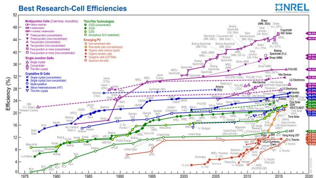
Fig.2. Best research-cell efficiency timeline (enlarge digitally to see details) (NREL 2016).
