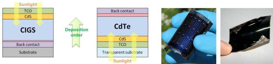
Fig.4. Principle configuration build-up and photos of flexible CIGS (nos. 1 and 3 from left) and CdTe (nos. 2 and 4 from left) thin film solar cells (Buecheler et al. 2011).
