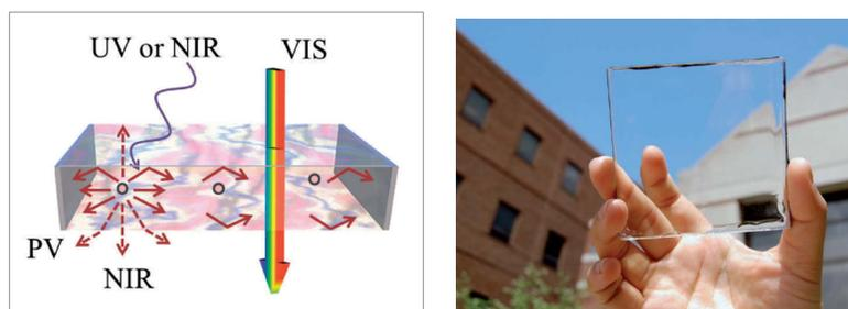
Fig.3. Solar harvesting tuned to absorb specific non-visible wavelengths of solar radiation and letting visible solar radiation pass straight through (Mourant 2014).
