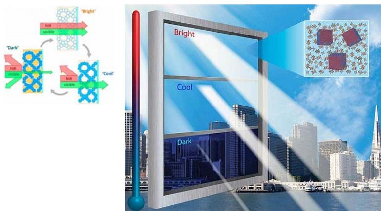
For a new habitation, Solar vacuum tubes collector is integrated in facade and covered by a smart dynamic glass as electrochromic glass with control of glass transparency. This system is used to control solar energy according to seasons with high insolation and heat requirements. PV modules can be installed to control electrochromic glass.
