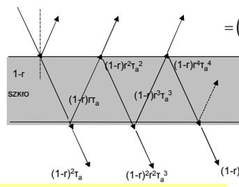
$$\tau_s = (1-r_s)^2 \tau_a + (1-r_s)^2 r_s^2 \tau_a^3 + (1-r_s)^2 r_s^4 \tau_a^5 + (1-r_s)^2 r_s^6 \tau_a^7 + \dots =$$
