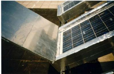
Effective use of diffuse booster reflectors to PV and PV/T systems to improve performance
