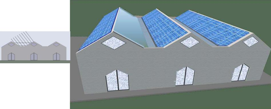
Building roofs can be effectively used to install PV modules, filling the opposite roof surface with diffuse reflectors, to provide additional solar energy and increasing system's electrical output
