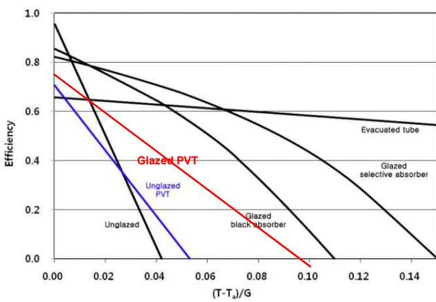
Comparison of thermal efficiency curves of solar thermal and PV/T collectors
