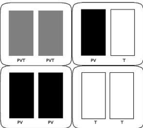
An effective system is the thermal collectors with PV/T collectors connected with the same water storage tank. The PV/T collectors preheat the water and the thermal collector s work for the main heating.
