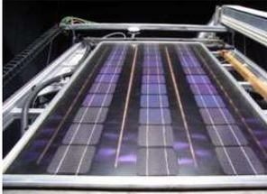
RenOn : PV cells attached on thermal absorber
