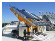
Fig.1 : Outdoor tracking device with solar air heater test stand at TestLab Solar Thermal Systems of Fraunhofer ISE
