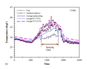
The experimental results during application of the solar chimney and water spraying during July
