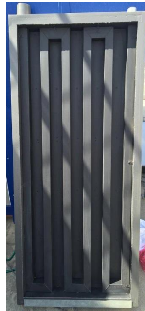
Figure 4.6. Painting black the integrated hot air collector with a mild steel square tube duct
