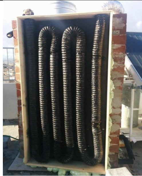
Figure 4.4. Positioning the aluminium foil duct in the integrated hot air collector utilising an aluminium foil duct
