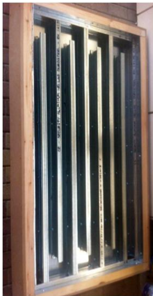
Figure 4.5. Fixing the internal metal separators in the integrated hot water collector with internal metal separators
