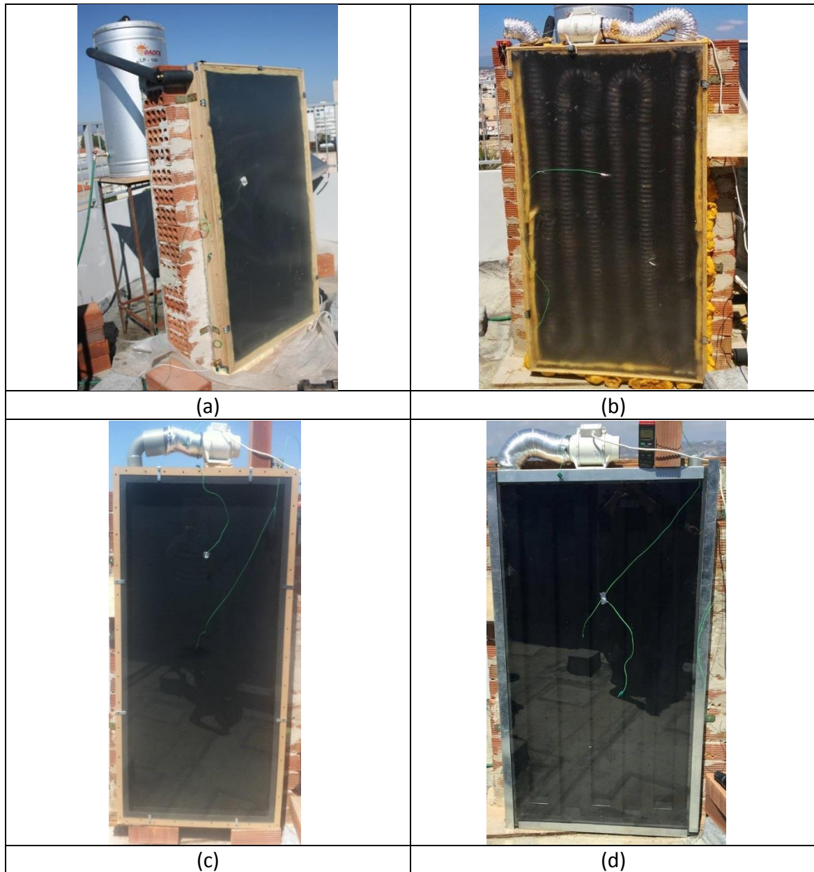
Figure 4.2: Prototype constructions, (a) integrated hot water collector (b) integrated hot air collector utilising an aluminium foil duct (c) integrated hot air collector with internal metal separators (d) integrated hot air collector with a mild steel square tube duct.
