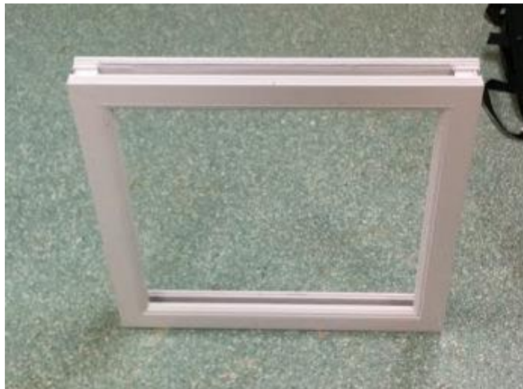
Figure 5.4. The UPVC window frame used to mount the glazing. Slots on the upper and lower sections allow for the air to flow through the glazing cavity.
