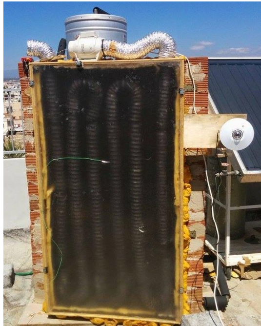
Figure 4.7. Pyranometer, air flow meter and temperature sensors in position for testing the performance of the integrated hot air collector utilising an aluminium foil duct.
