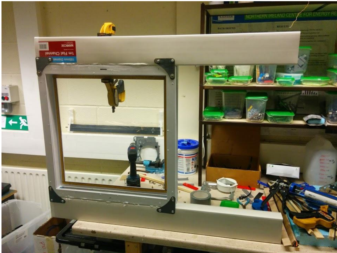
Figure 5.5. The inlet and outlet header air ducts attached on the UPVC window frame.
