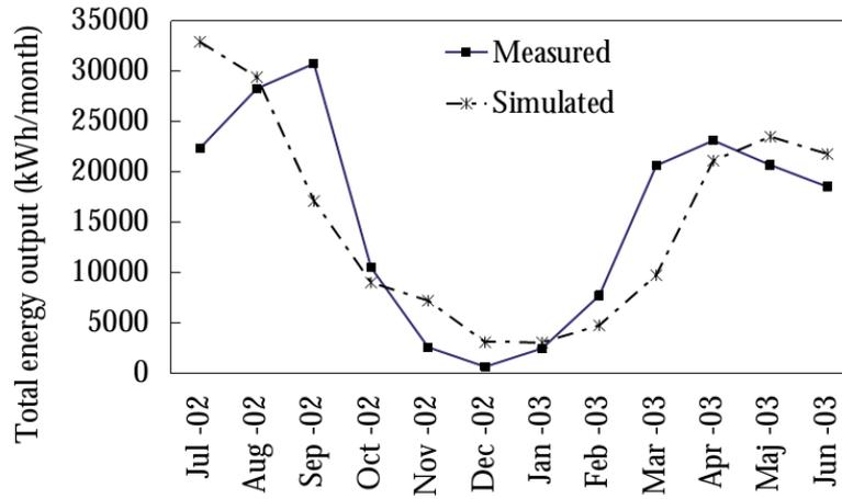
Figure 15 Measured and simulated results of the total monthly energy output from the solar thermal system.
