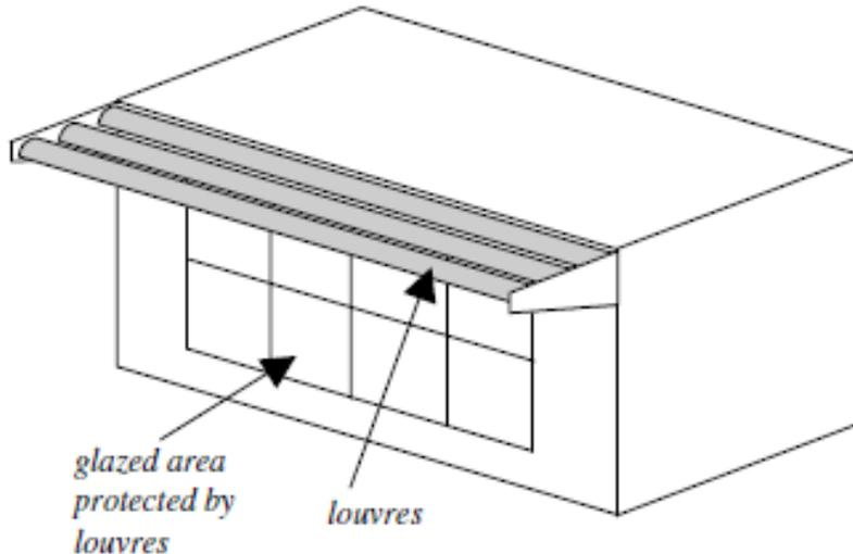
Figure 4.1 Use of a solar louvers collector to protect glazed surfaces (Palmero and Oliveira, 2006).
