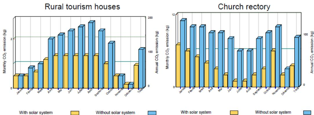
Figure 6.10 Avoided CO<sub>2</sub> emissions for the vacuum solar collector H2OSS.
