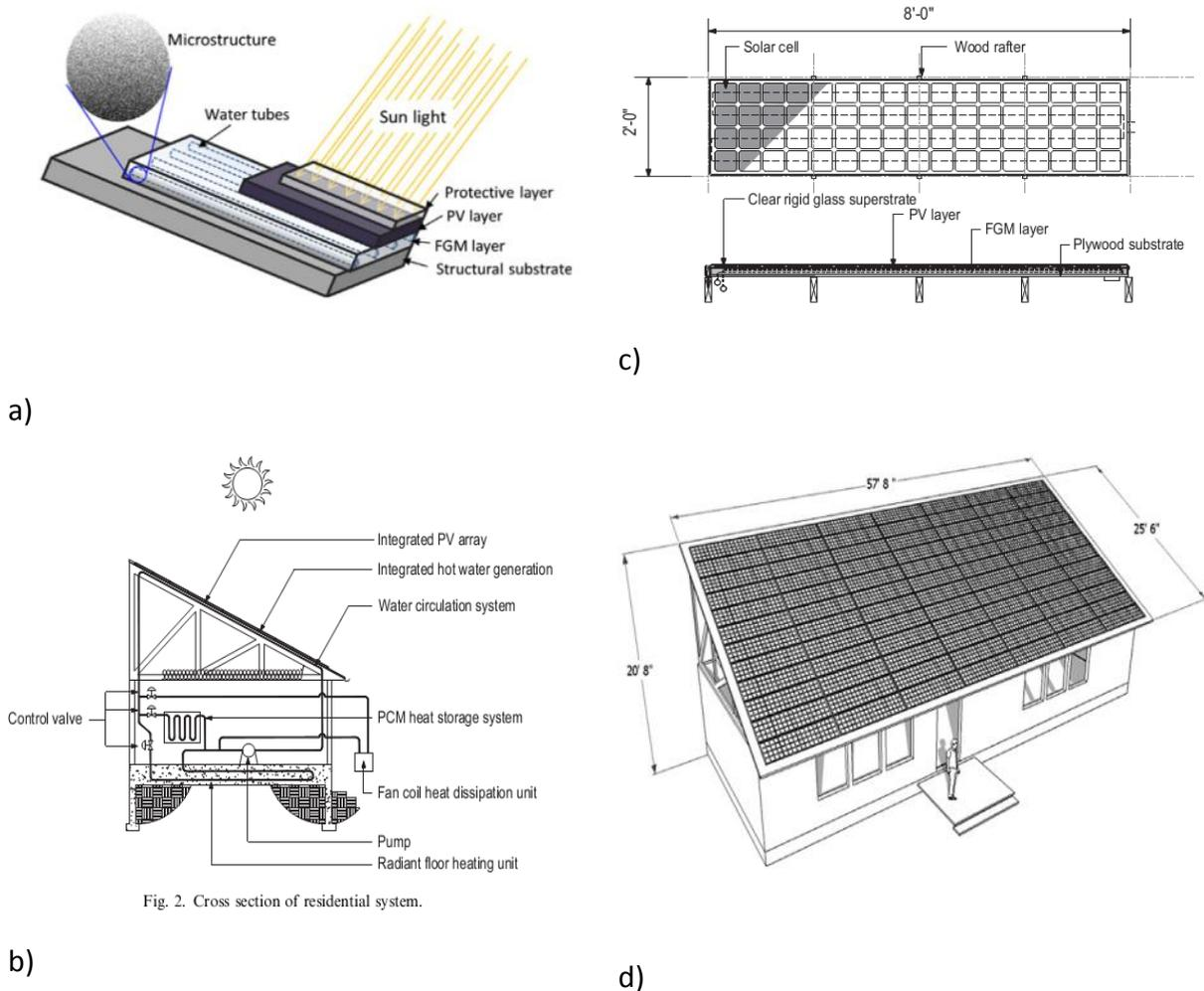
Fig. 2. Cross section of residential system.
