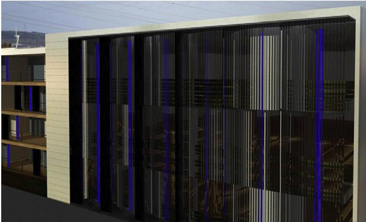
*Figure 4.5 Architectural design of the building integrated concentrating system. The blue lines behind the Fresnel reflectors indicate the position of the receptors which are installed on the facade (Chemisana et al., 2013).*
