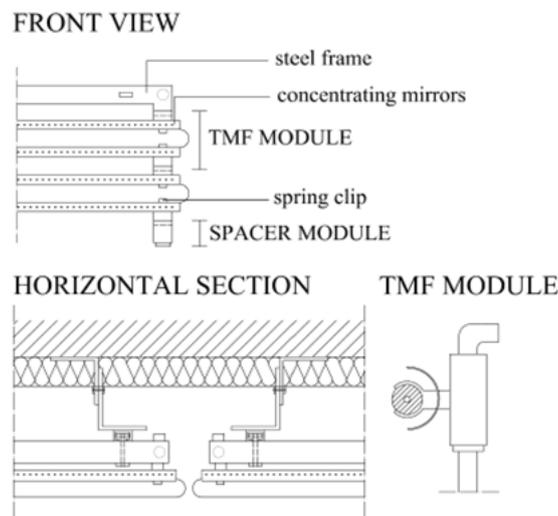
Figure 7.11 Design of a panel made by Tube mirror frame module.
