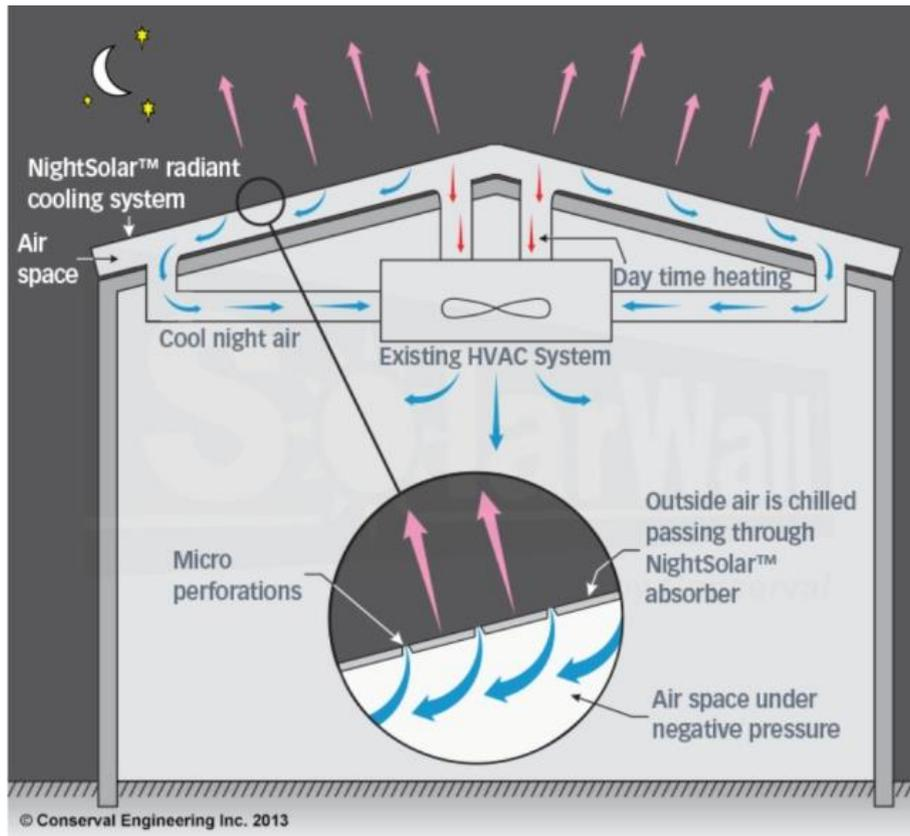
Figure 3.4 NightSolar® system showing the principle of operation.
