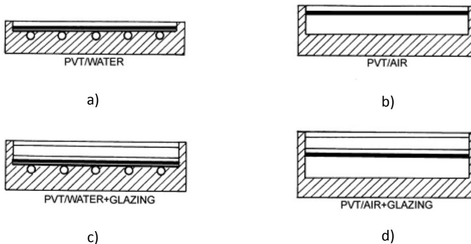
Figure 5.1 Cross section of the main PV/T geometries, a) PVT/water (unglazed) b) PVT/air (unglazed) c) PVT/water with glazing d) PVT/air with glazing.
