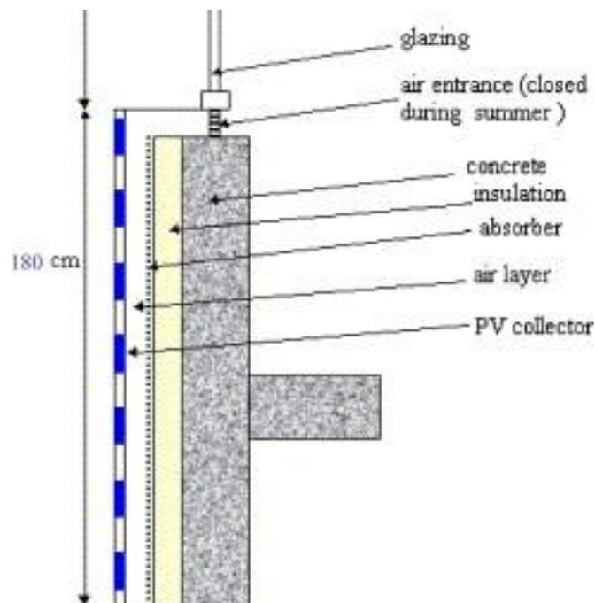
Figure 4.2 PV collector integrated in the facade, side view (semi-transparent PV collector preheating the ventilation air) (Guiavarch and Peiportier, 2006).
