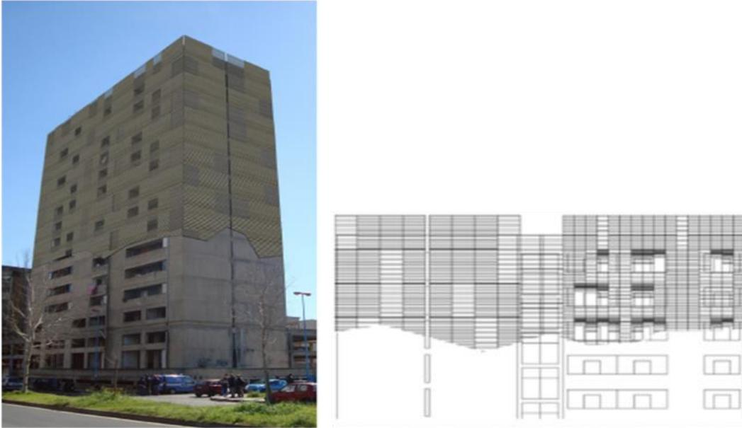
Figure 12.7 Proposed Building – Current façade and simulation of the new proposed solar thermal cover.
