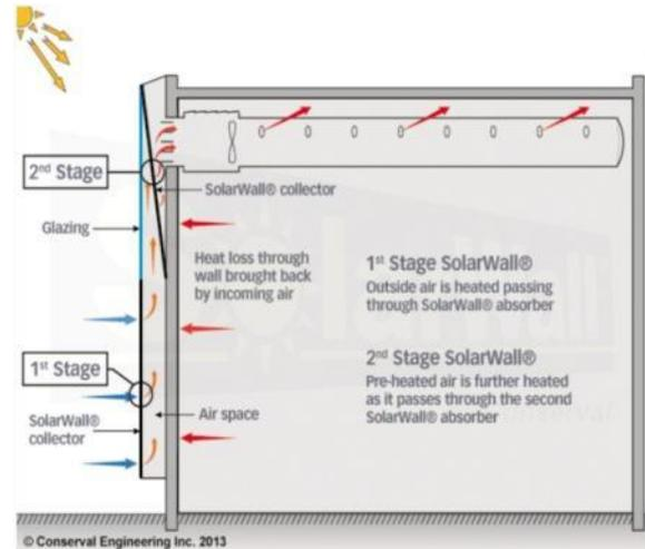
Figure 3.2 2-Stage SolarWall patented system® with Interior Fan.
