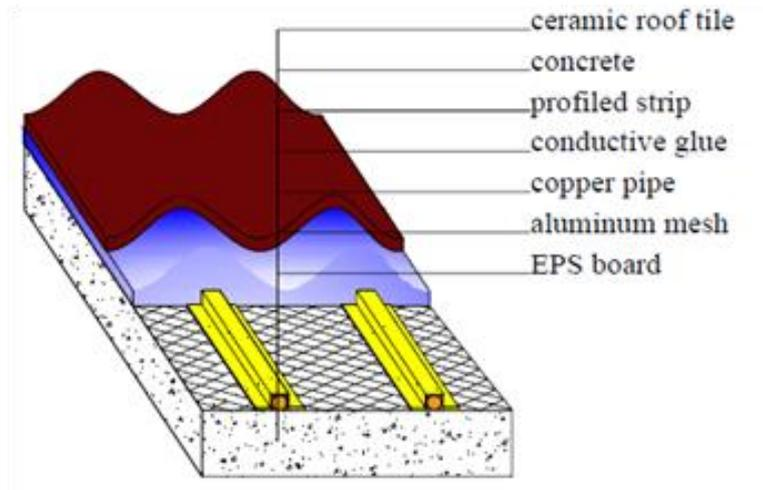
Figure 7.2 The arrangement of the solar collector.
