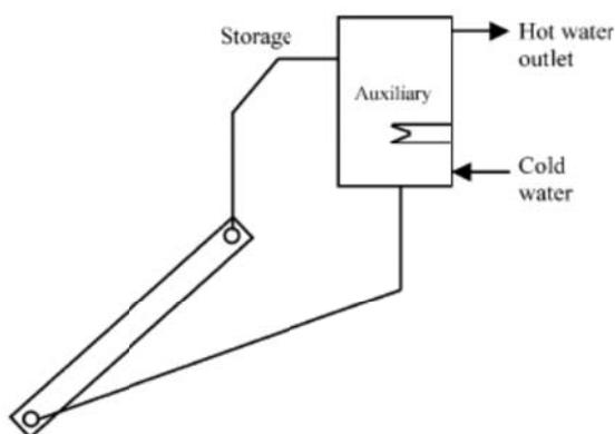
Figure 3-4 : Simple schematic of the thermosiphon system
