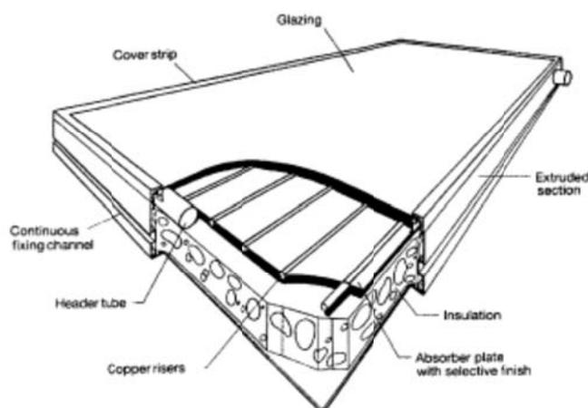
Figure 3-1: Typical Flat Plate collector (Kalogirou 2004)
