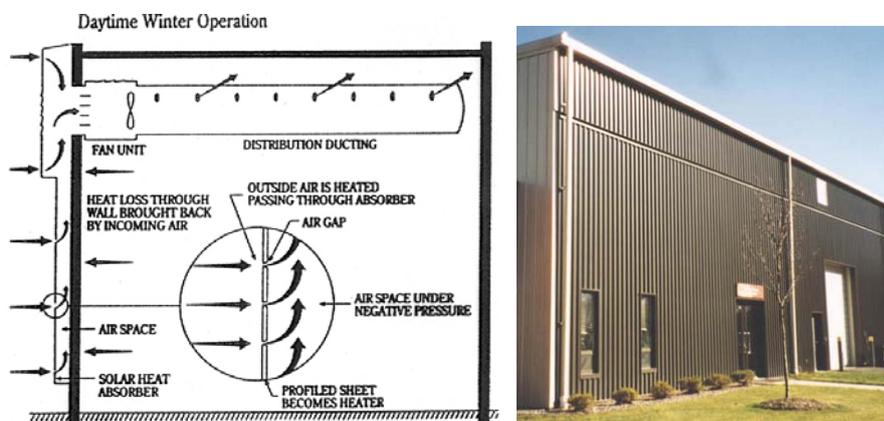
Figure 4.12. Construction as conventional façade cover, (SolarWall 2014)
