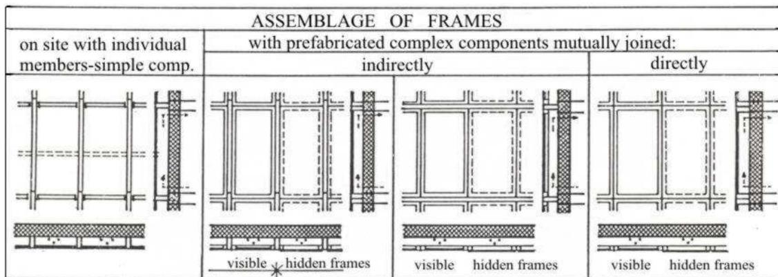
Figure 4.9. Suspended façade assemblage possibilities (Krstic-Furundzic 2007)
