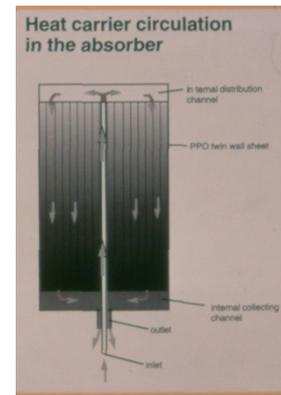
Figure 4.7. Building integrated STC made of polycarbonate twin wall absorber sheet filled with ceramic particles.
