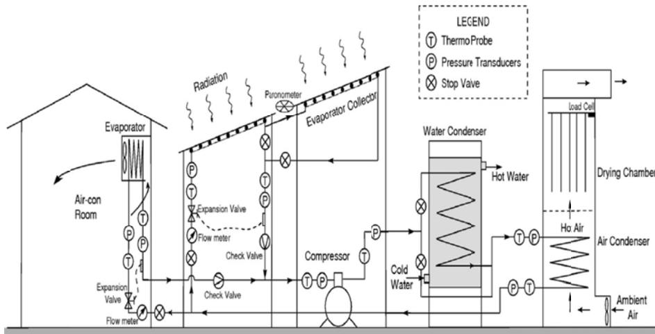
Figure 3-12 : Schematic diagram of a roof integrated (integral) solar heat-pump system (Zakaria, Hawlader 2013)
