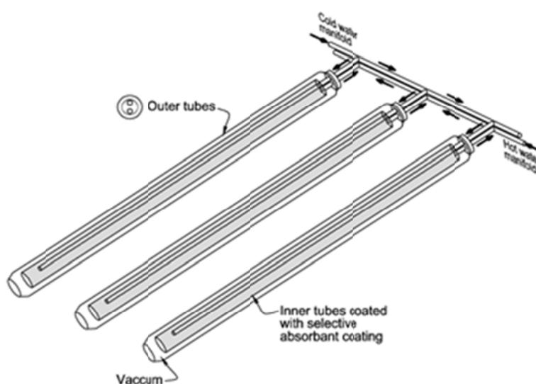
Figure 3-3 : Metal/glass water pipe evacuated tube solar collector
