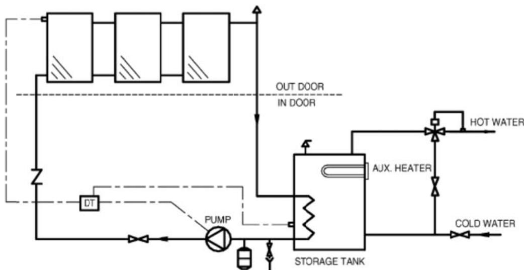
Figure 3-6 : Closed pressurized system (Kalogirou 2004)
