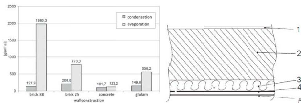
Figure 5-2. (left) Annual condensation and evaporation potential for different wall constructions, (Bergmann, Weiss 2002). (right) Wall constructions: (1): interior plaster, (2): brick 38cm / brick 25cm / concrete, (3): insulation, (4): absorber, (5): glazing (Similar configuration for “glulam” with more wooden layers) source (Bergmann, Weiss 2002).
