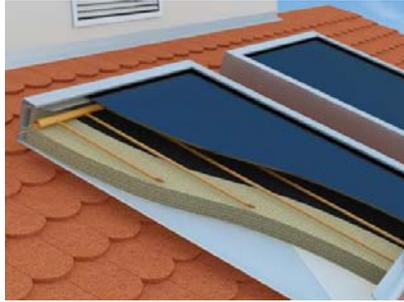
Figure 5.1. Solar panel thermal insulation (Canada Mortgage and Housing Corporation 2014)
