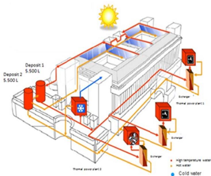
Figure 3-10 : A BISTS for hot water production with centralized storage and heating and cooling (via absorption chiller) (URBAN SOL PLUS 2008)
