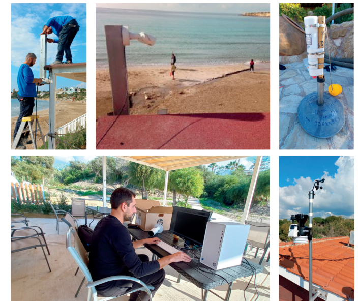
Coastal monitoring system (camera installation, meteorological station and wave sensor)
