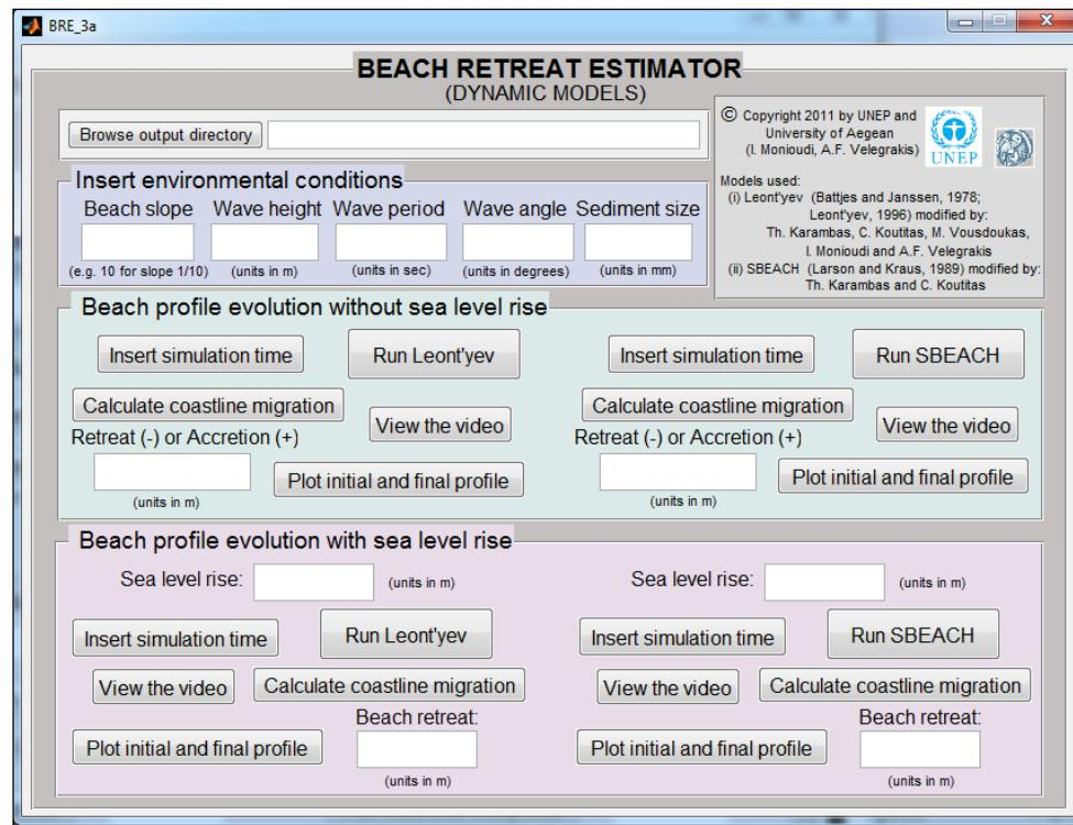
**Figure 1.** The figure of the BRE\_3a GUI (for linear profiles).
