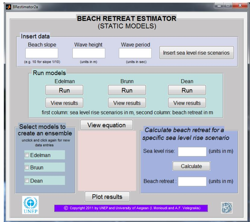
**Figure 1.** The figure of the BRE\_2a GUI (for linear profiles).
