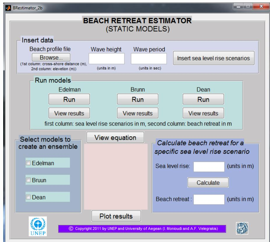
**Figure 2.** The figure of the BRE\_2b GUI (for natural profiles).
